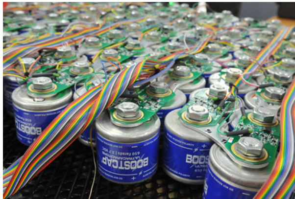
Figure 5: Supercapacitor pack with Maxwell Boostcaps (Source: Argonne National Laboratory)
