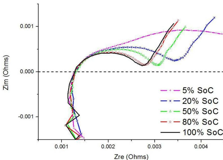
Figure 3: Comparison of EIS response at various SoC (from [7])
