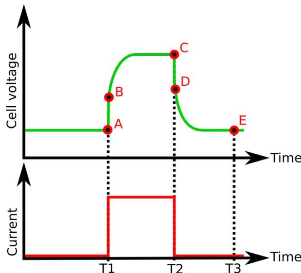
Figure 2: Current step response of a cell
