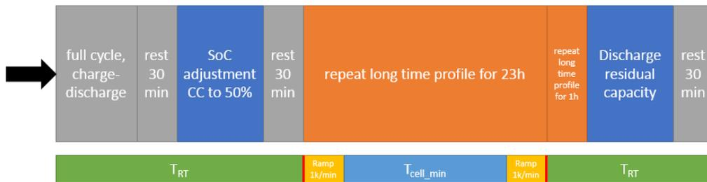
**Figure 8: SoC validation with 24h long time profile at  $T_{cell\_min}$**
